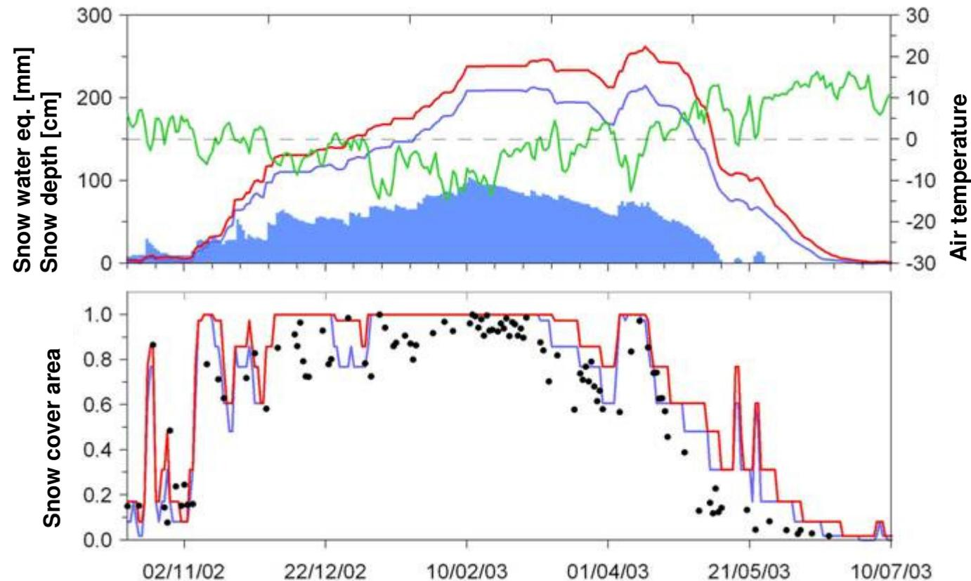
Rainfall-runoff model with threshold air temperature used for snow accumulation and degree-days used for snowmelt
