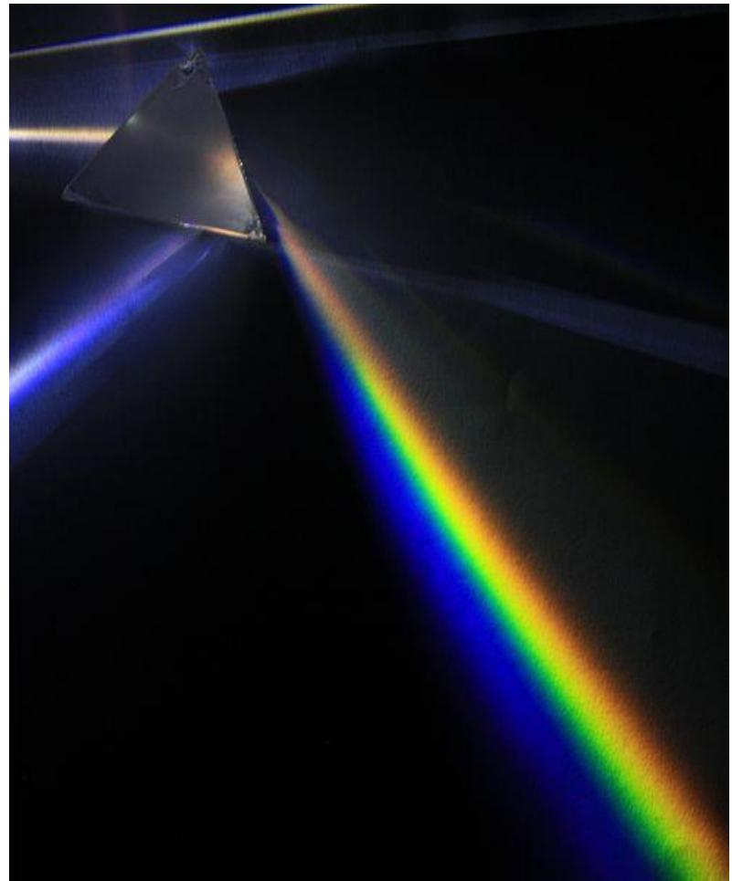
White light from a Mercury vapour lamp passed through a flint glass prism.
